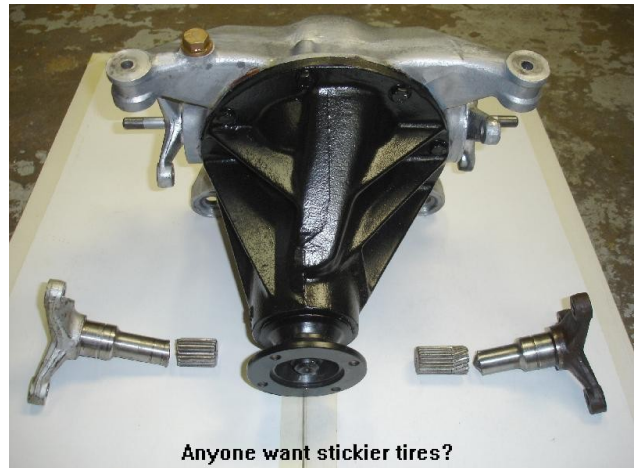
Detail of Circlip Groove Repair - beautiful but expensive
